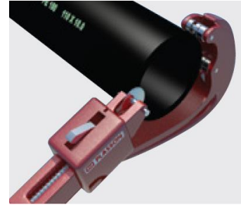
Figure X-a – Cut Pipe Ends
