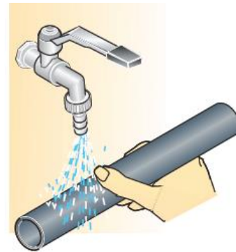
Figure X-b – Clean Pipe Ends
